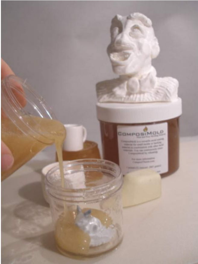
CompositMold Mold Making Material being used to mold a small rabbit figurine with other examples of parts cast in CompositMold Molds.
